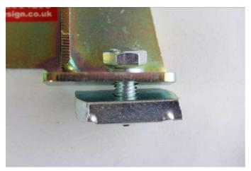
You can probably see how the brackets fit- they sit on top of the raised lips on your van with the threaded nut plate underneath the lip and an M8 bolt and spring washer through
